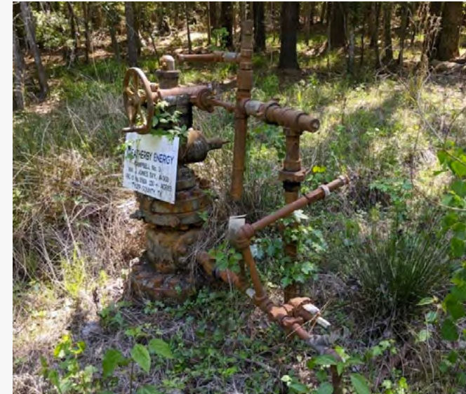
Federal funding is being used to plug orphaned oil wells in Big Thicket National Preserve/NPS file
